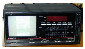
Sure enough on inspection with the oscilloscope at home, one set of coils showed a large waveform and the other almost nothing at all. I followed the wires back to the PCB and the PCB traces back to the driving transistor and it was clear the amplitude of the signal on its collector was a lot smaller than the base signal.
