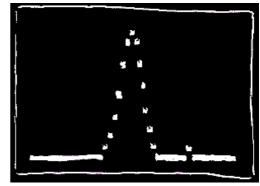
Following that it is simple to arrange for frequency sweeps to alternate between each input channel, writing into successive 512-byte blocks of memory. Both channels will share the same frequency sweep range. The sweep rate is thereby halved from 25 sweeps per second to 12.5.
