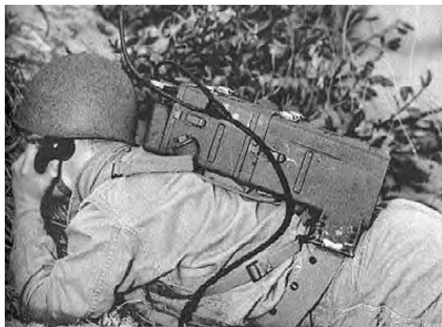
Figure 38-4 SCR-300 on back of soldier. Whip has semi-rigid base to allow vertical positioning. Bottom 3/5 of case is batteries.
