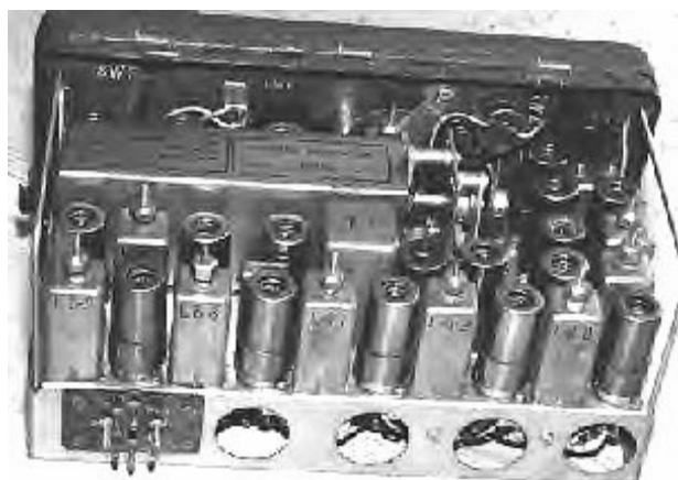
Figure 38-6 Rear view of the BC-1000 R/T chassis. Tuning capacitor shield is long box structure at middle-left. All tubes have shields holding them in place.
