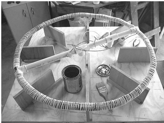
Figure 39-13 Wire bundle is cord-wrapped and ready for varnishing.
