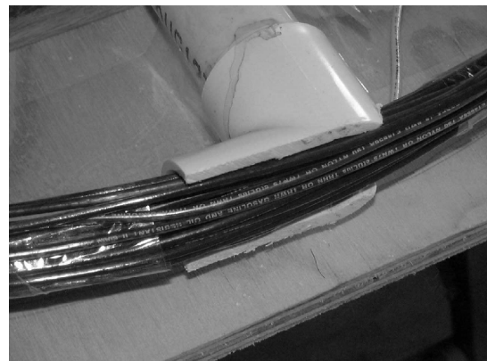
Figure 39-10 Wire lays nicely into the modified right-angle pieces. Strips of transparent shipping tape have been used for temporary wire bundle holds.
