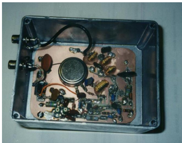
A varactor tuned 5 MHz VFO. Tuning is accomplished with the big round potentiometer.
