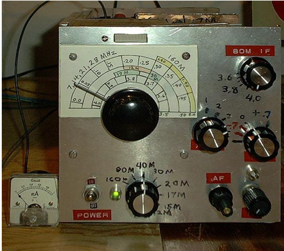
Homebuilt all-band dual conversion HF ham receiver.
