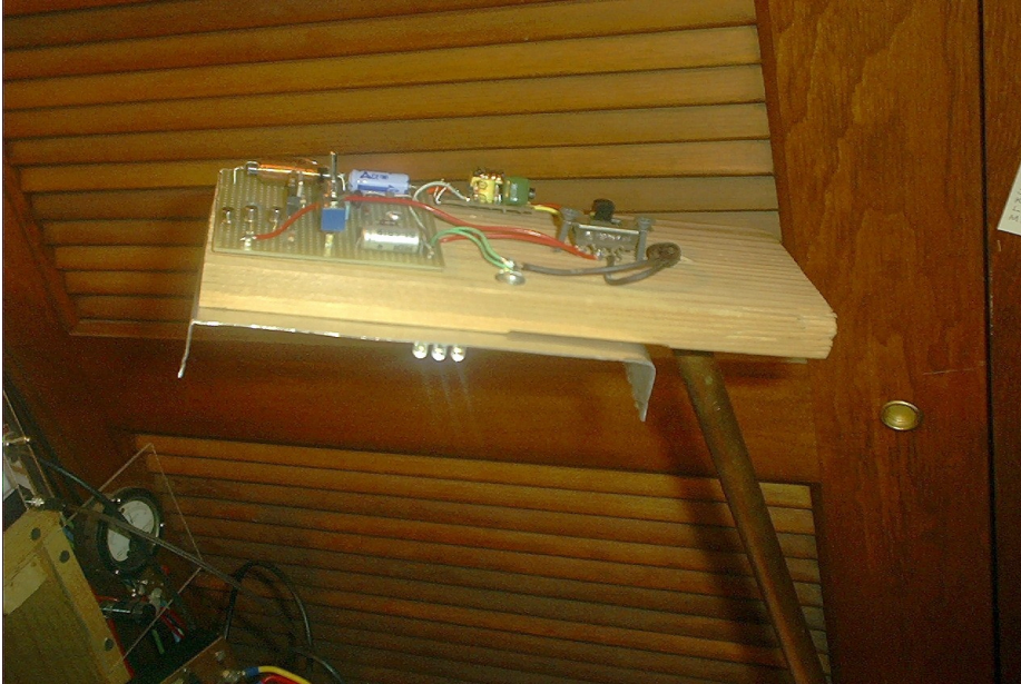
A homebrew LED and fluorescent station lamp
